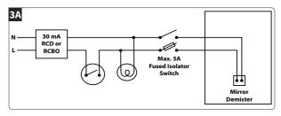
The Warmup Mirror Demister can be connected into the rooms lighting circuit, enabling the demister when the lights are switched on.
