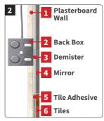
Ensure when mounting the mirror that the supply cable and its connections are not trapped behind the mirror, which would cause the mirror to be stressed or sit unevenly on the wall.
